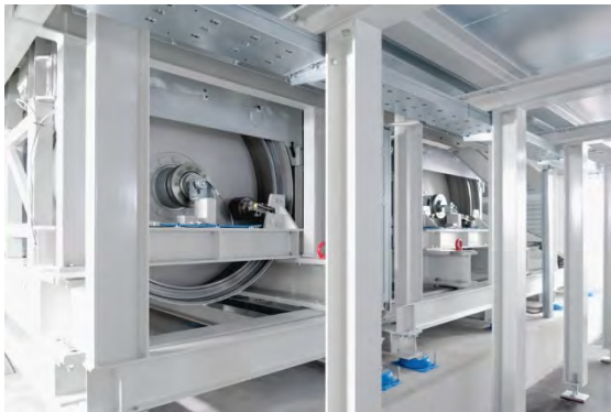
Integral Powertrain installed Horiba Vulcan II Xtra Cold Dynamometer
